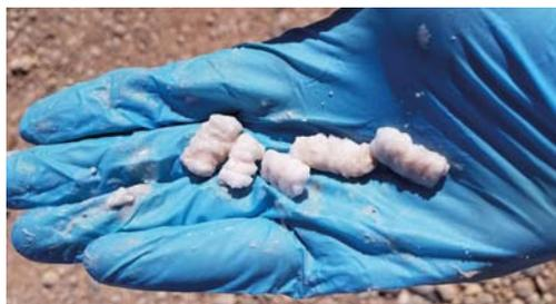
The direct emulsion system performed with no phase separation of the oil and brine phases despite numerous drilling challenges. Cuttings through the salt showed no sign of dissolution (left).
