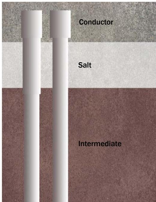
EnerSEAL enabled drilling the salt layer and intermediate sections in a single casing run. The original design (above, left) required five extra days to drill as compared to the new casing design (above, right) after the introduction of EnerSEAL.
