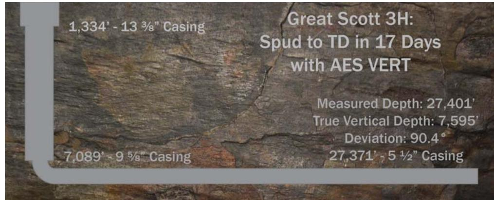
Eclipse Resources is drilling multiple horizontal wells with laterals exceeding 19,000 feet using AES VERT. Extended laterals are critical to efficient production delivery in the Utica shale of Eastern Ohio.
