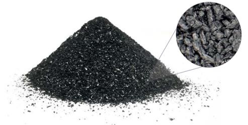
Under pressure, ENER-GS has the ability to compress and exhibit a resiliency that allows it to remain closely packed within fractures and pores across a wide range of drilling fluid densities and temperatures.
