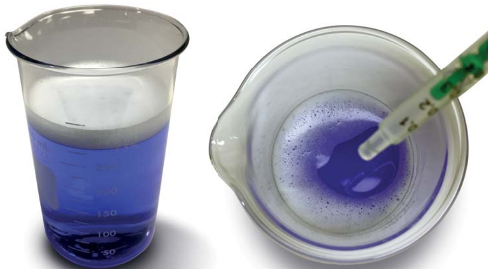
Foam sample prior to (left) and after ENERDEFOAM treatment (right) Note: base fluid color added for contrast
