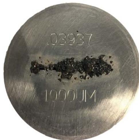
In this example slot test, 20 lb/bbl ENERLOC was added to an unweighted invert emulsion to seal the 1000 micron slot sealed at 500 psi
