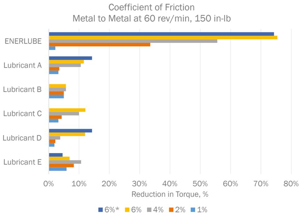
Coefficient of friction data comparison between ENERLUBE and competing lubricants across various concentrations. \*Reading after 16 hour hot roll at 250°F.
