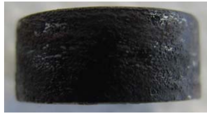
A corrosion test was performed comparing 10.4 lbm/gal calcium chloride brine with and without the EnerCLEAR corrosion package at a pH of 11. The untreated sample had an equivalent corrosion rate of nearly 100 mpy while the treated sample was less than 2 mpy.
