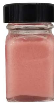
Invert Emulsion (typical OBM): Water droplets are dispersed in an oil-continuous phase
