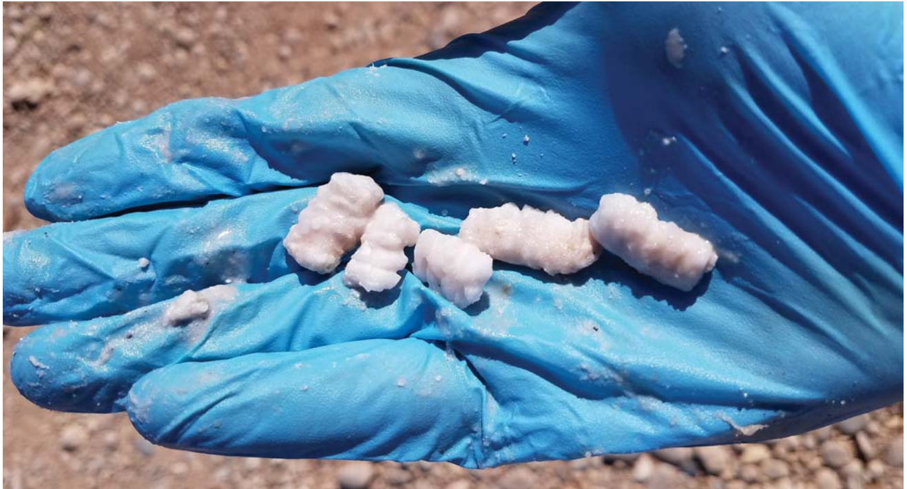
Salt cuttings from the shakers indicate complete inhibition with a 9.2 lbm/gal EnerLITE system.
