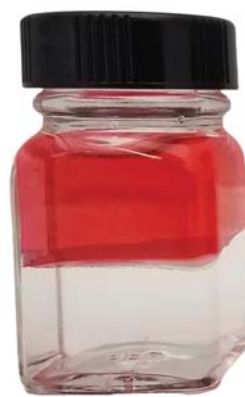
No Emulsion: In a normal state, oil and water do not mix.
