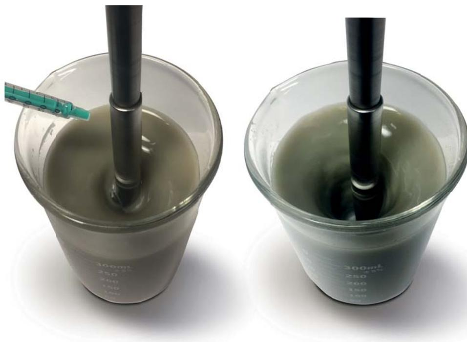
In a lab test, a sample contaminated with shale is treated with KCL SUBSTITUTE (left). As a potassium chloride substitute, KCL SUBSTITUTE efficiently reduces shale hydration (right). Note the larger vortex as reactive clay is inhibited, thinning the fluid sample.
