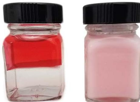
Diesel and water (left) quickly separate. NORMUL stabilizes the EnerLITE direct emulsion system (right) to maintain an oil-in-water emulsion.
