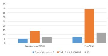
Conventional MMH versus EnerSEAL Contaminated with 0.25 lb/bbl Lignite
