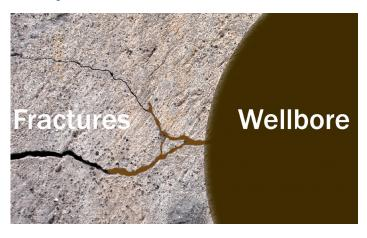
**Figure 3.** EnerSEAL enters the low shear region of a fracture network, thickening and slowing or eliminating losses.
