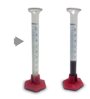
In a lab test, a clay contaminated water-based fluid demonstrated high API fluid loss (left). A treatment of 0.50 lb/bbl DEFLOC 2000 dramatically reduced fluid loss (right).
