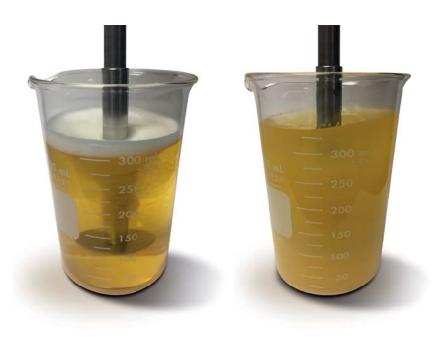
In a lab test, a sample demonstrated high foaming tendencies (left). A treatment of 0.1 lb/bbl DEFOAM A dramatically reduced foaming (right).
