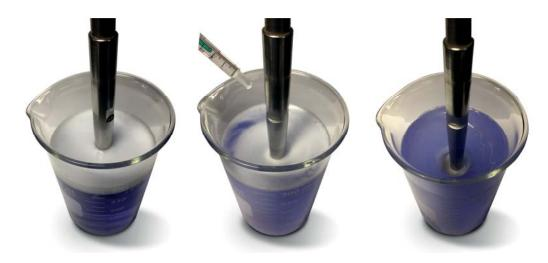
In a lab test, a sample demonstrated high foaming tendencies (left). A treatment of 0.05 lb/bbl DEFOAMEX SB dramatically reduced foaming (Center and right).
