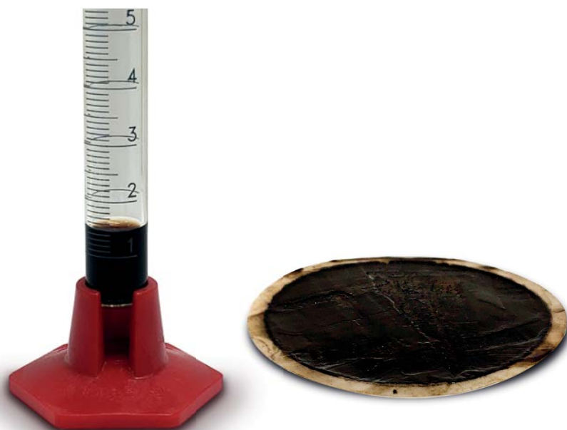
Filtercake (right) and filtrate (left) of an oil based fluid system using DURATEC ER at 300°F. As part of a properly designed system, DURATEC ER provides excellent filtration control.
