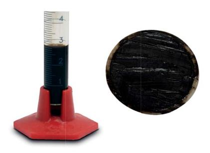
Filtrate (right) and filter cake (left) of an invert emulsion system featuring DURATEC at 250°F. As part of a properly designed system, DURATEC provides excellent filtration control.
