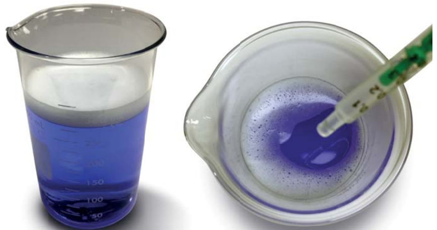
Foam sample prior to (left) and after ENERDEFOAM treatment (right) Note: base fluid color added for contrast
