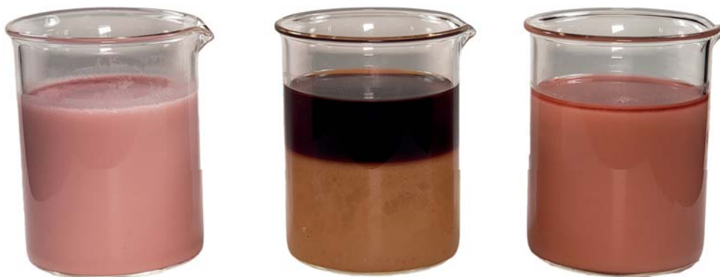
Compatibility comparison of untreated EnerLITE (left), EnerLITE with a conventional lubricant (center), and EnerLITE treated with ENERLUBE LITE (right).
