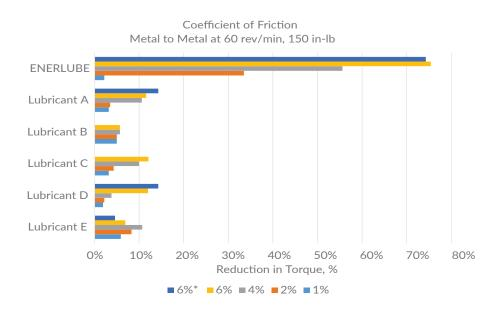
Coefficient of friction data comparison between ENERLUBE and competing lubricants across various concentrations.
