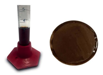
Filter cake (right) and filtrate (left) of EnerREACH system using ENERMUL II as secondary emulsifier at 250°F. As part of a properly designed EnerREACH system, ENERMUL II provides tighter filtration control and emulsion stability.
