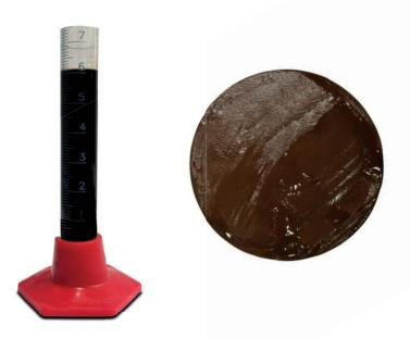
Filtrate (left) and filter cake (right) of EnerREACH system using ENER-MUL at 300°F. As part of a properly designed EnerREACH system, ENERMUL provides excellent filtration control and emulsion stability
