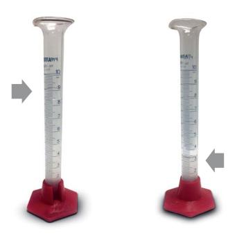
In a lab test, a clay contaminated water based drilling system demonstrated extremely high API fluid loss (left). A treatment of 1.25 lb/bbl ENERPAC R dramatically reduced fluid loss (right)
