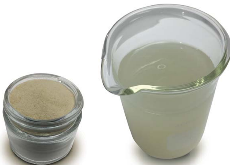
ENERZAN sample (left) and viscous fluid containing 2 lb/bbl ENERZAN dispersed in water (right)
