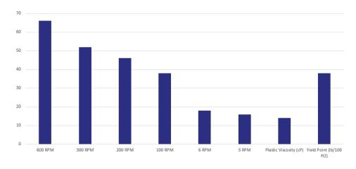
EnerSEAL example rheological profile measured at 120°F during a drilling application when used in conjunction with ES-VIS at a 10:1 ratio of ES-VIS to ES-RM
