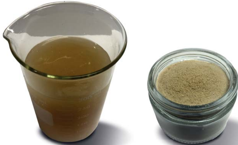
XG-VIS rheological modifier blended in freshwater (left) and product (right)
