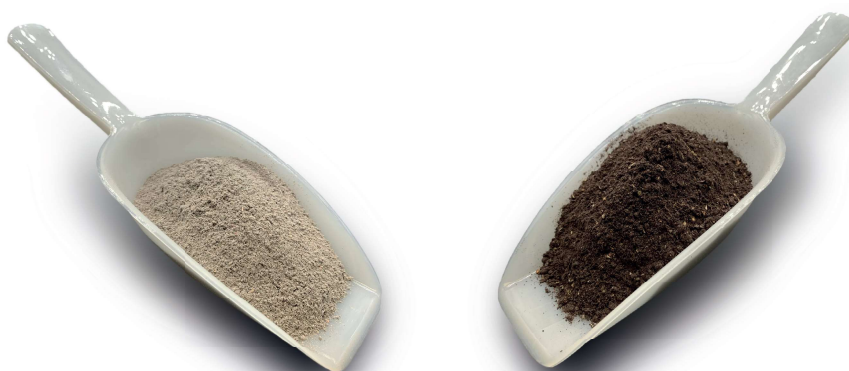
ECM 1 (left) and ECM 2 (right) provide an optimized particle size distribution for treatment of lost circulation
