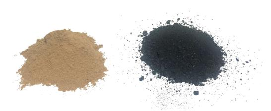
EOSEAL II (left) is a proprietary blend of cellulose fiber and polymer and ENERLOC (right) is a blend of granular and fibrous materials. Both blends are designed to address losses in challenging environments where typical lost circulation products fail.
