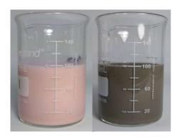
Fresh EnerLITE (left) features an initial mud weight that increases as drilled solids are incorporated into the system (right).
