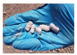
The direct emulsion system performed with no emulsion instability despite numerous drilling challenges. Cuttings through the salt showed no sign of dissolution (left).
