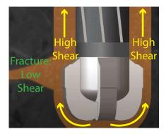
EnerSEAL mitigates losses as it becomes thicker at low shear, such as near fractures, slowing or eliminating lost circulation in troublesome zones such as the Brushy Canyon and Cherry Canyon formations
