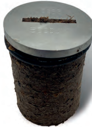
MACRO STRENGTH High Fluid Loss Squeeze Material plugging a 5000 \mu slot
