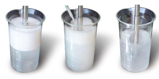
In this lab test, a brine sample demonstrates high foaming tendencies (left). A treatment of 0.05 lb/bbl DEFOAMEX SB II dramatically reduces foaming (center and right).
