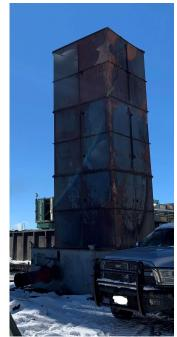
Figure 5: Self-contained flare stack
