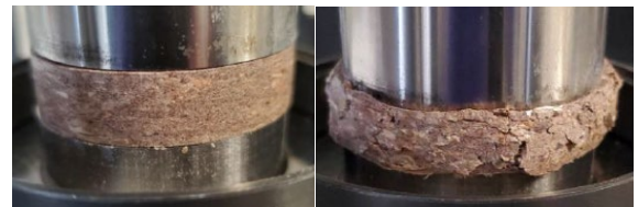
Figure 6 – UCS testing performed on an optimized HFLS blend, the left image illustrating the material before deformation, and right picture illustrating the material after deformation
