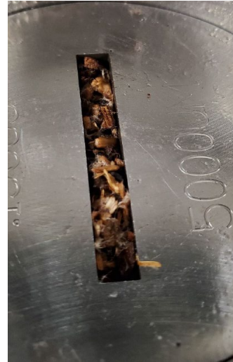
Figure 5 – Base fluid of the HFLS experimental blend after applying 1,000 psi across a 5,000 micron slotted disk
