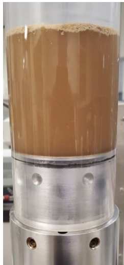
Figure 4 – Base fluid of the HFLS experimental blend after applying 1,000 psi across a 5,000 micron slotted disk
