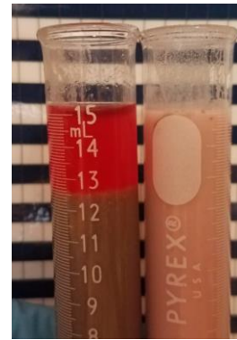
Image 6: Bench top centrifuged samples during saltwater flow (left) and prior to drilling (right)
