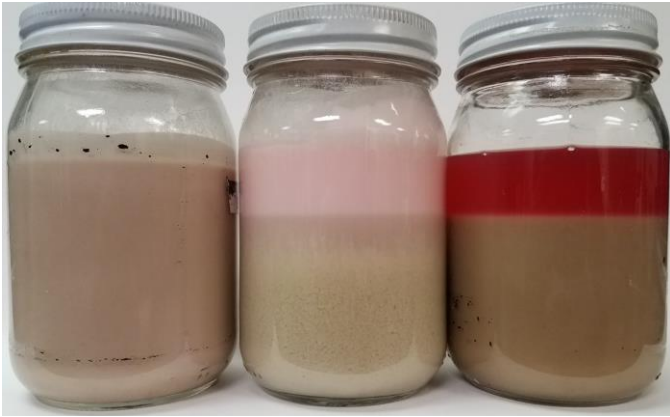
Image 2: Successful sample (left), emulsified phase separation (center), and top-oil separation (right)
