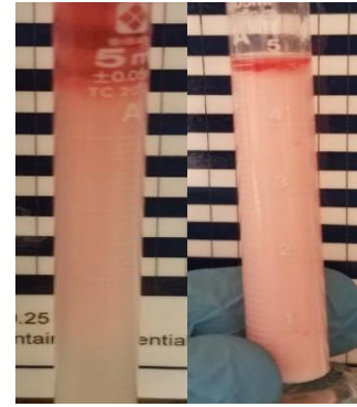
Image 7: Filtrate where system requires treatment (left), system response to treatment (right)
