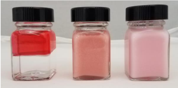
Image 1: No emulsion (left), 70:30 oil:water ratio invert emulsion (center), and 30:70 oil:water ratio direct emulsion (right)
