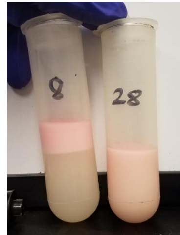
Image 4: Formulation #8 (left) and final formulation #28 (right) after bench top centrifuge
