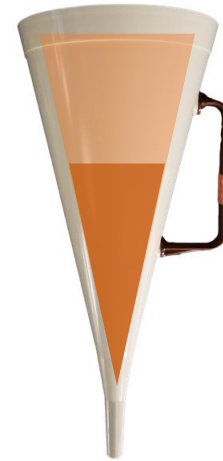
Figure 4: The Marsh funnel has a constantly changing rate of hydrostatic pressures and shear as fluid passes through, making it a poor instrument for precision measurements
