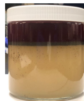
Figure 4: Broken emulsion following breaker treatment
