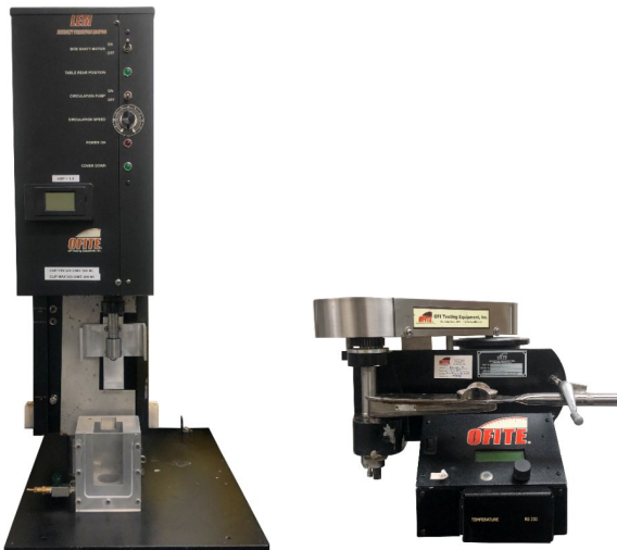
Figure 5 & 6 – The LEM (left) and Lubricity Meter (right) were the primary lab equipment machinery used to evaluate candidate lubricants
