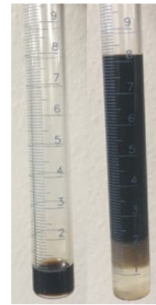
Figure 10 – 30 min. HTHP Fluid Loss Results at 250°F on Baseline OBM (left) and OBM with 3%/vol. Experimental Solvent 4 (right), indicating emulsion destabilization
