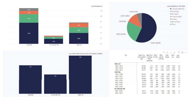
Figure 4. Dashboard visualisation comparing drilling fluid losses across 12 wells drilled by 3 rigs.
