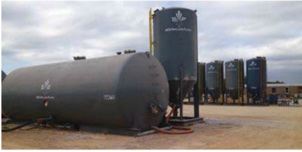
Figure 1. Bulk barite storage tanks in Pleasanton, Texas.
