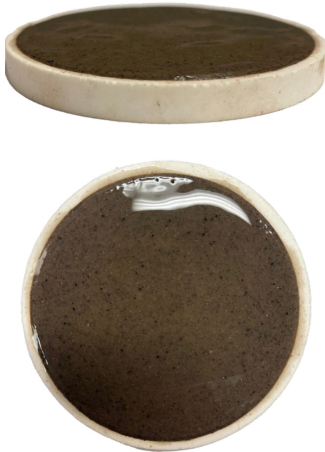
Figure 4. Filter cake generated by WALLPLEX on an aloxite disk.
