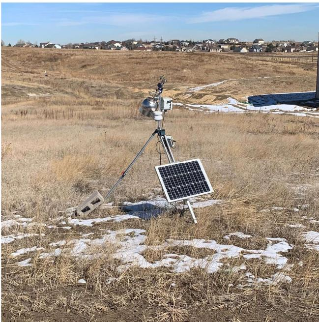
**Figure 4: Air quality and sound monitoring station – note the homes in the background of the image**
