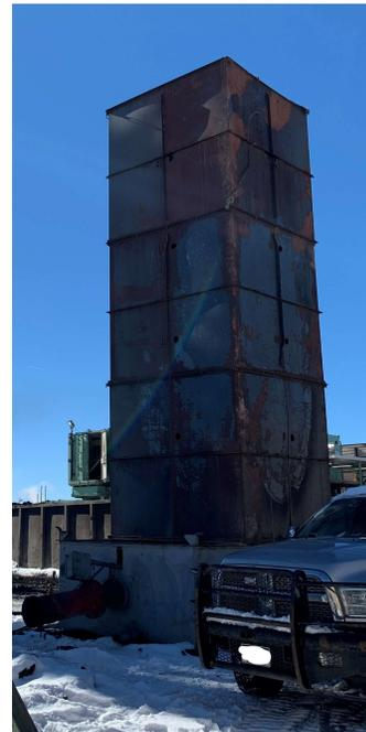
**Figure 5: Self-contained flare stack**
