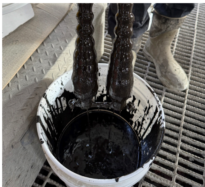
Figure 4. Magnet rod with metal debris attached after 1 hour circulation of 500 bbl used oil-based mud at the mix plant.
