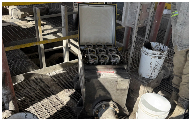
Figure 3. A total of nine magnet rods are positioned in the flow box, affixed above a 500 bbl mix pit at AES Drilling Fluids' wellsite in Kermit, Texas.
