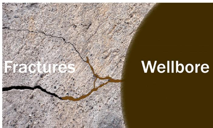
**Figure 3.** EnerSEAL enters the low shear region of a fracture network, thickening and slowing or eliminating losses.
