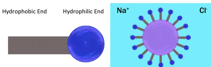
**Figure 4.** Left: A surfactant features a hydrophobic (oil-loving) tail and a hydrophilic (water-loving) head. Right: The new approach with the EnerLITE system was to feature a surfactant that created a stable dispersion of oil in saturated brine versus older freshwater systems.
