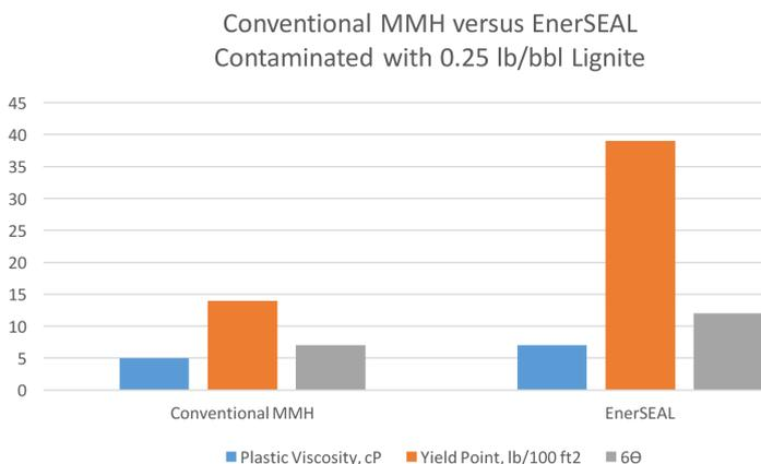
**Figure 2.** Conventional MMH versus EnerSEAL rheology at 120 °F with 0.25 lb/bbl of lignite.
