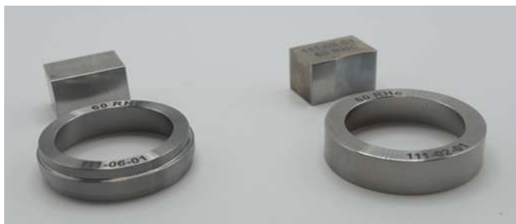
Figure 6. Image of the block and ring as part of the EP testing assembly (left) and an image of the block and ring as part of the standard lubricity tester (right). A torque wrench is utilised to apply pressure, forcing the block against the ring as it rotates, while immersed in a test solution.
