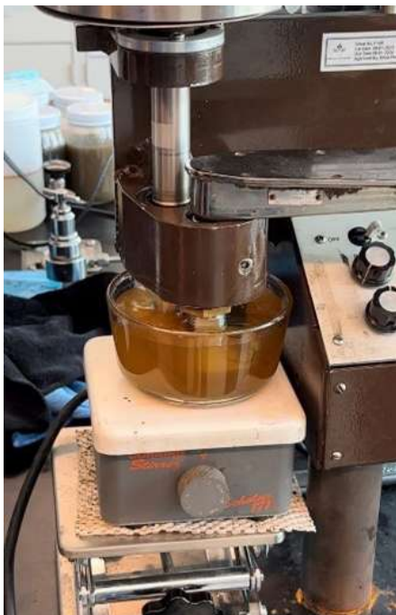
Figure 3. The modified extreme pressure lubricity tester includes a larger motor and stirring assembly to ensure proper lubricant dispersion during testing.
